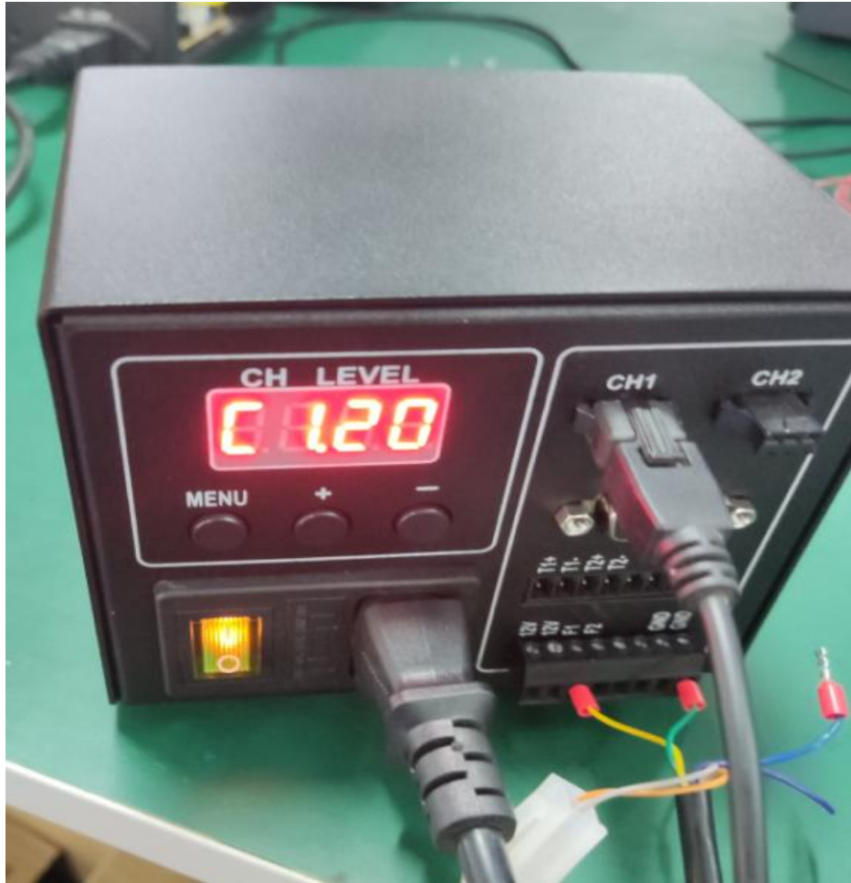
Figure 24: Set Trigger Signal Output Delay to 20 \mu s
