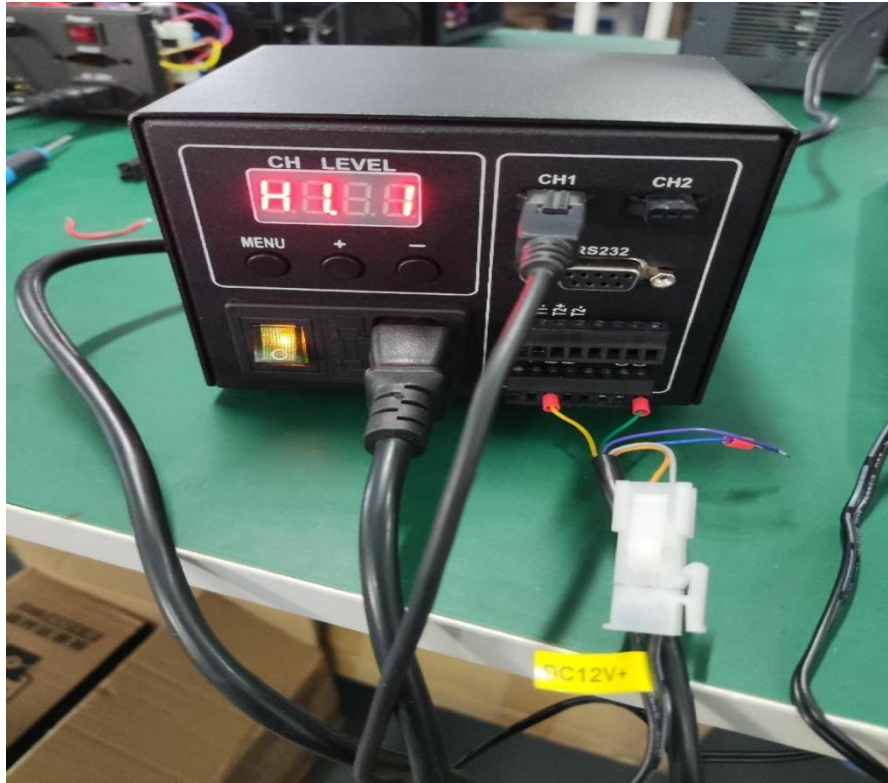
Figure 22: Set to Internal Trigger Mode
