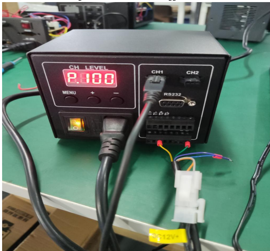
Figure 23: Set Internal Trigger Cycle to Trigger Once Every 100 ms
