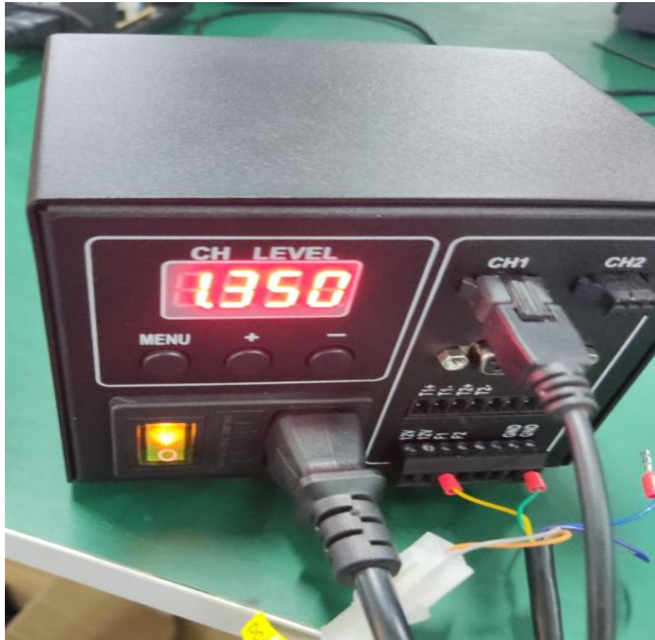
Figure 21: Strobe Time Setting and Wiring Method
