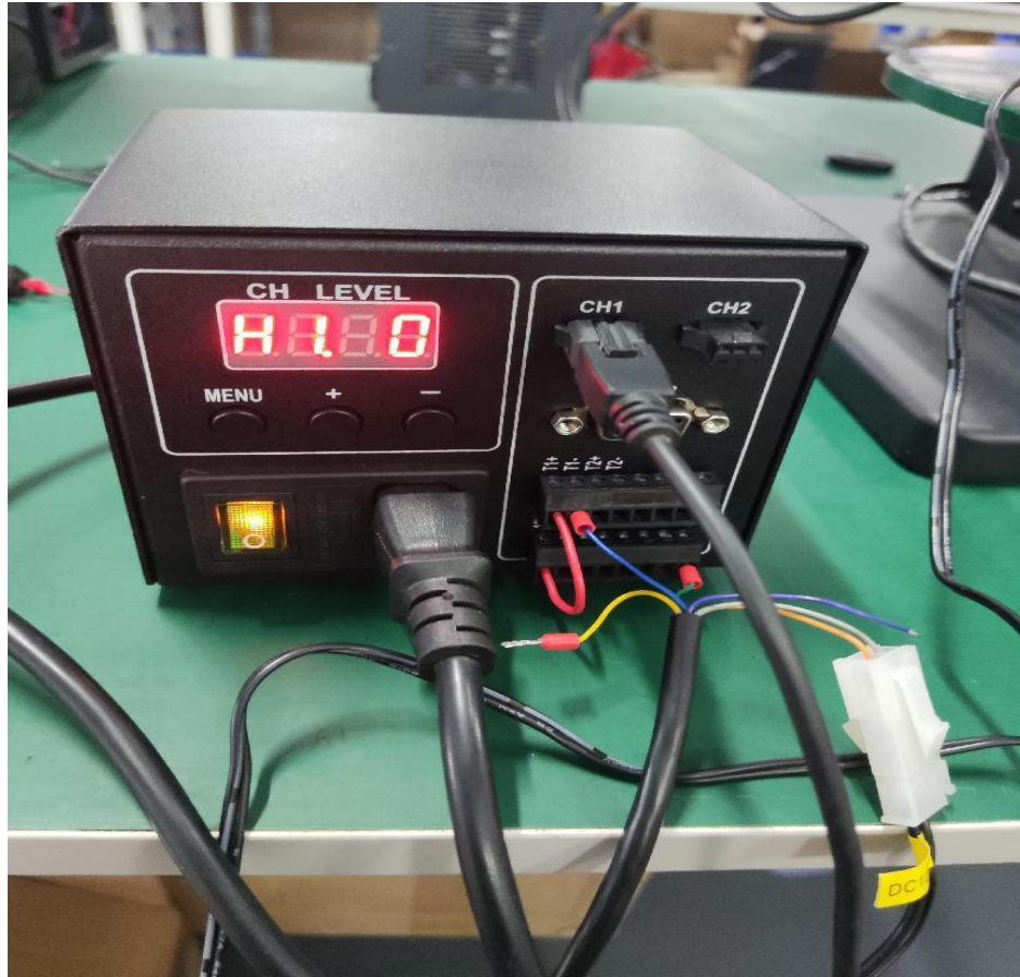
Figure 18: Set to External Trigger Mode
