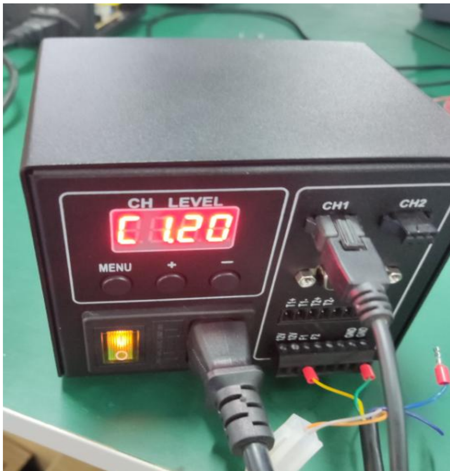
Figure 23: Set Trigger Signal Output Delay to 20 \mu s
