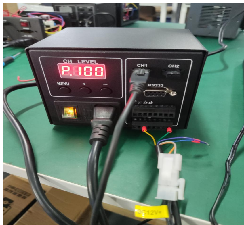
Figure 22: Set Internal Trigger Cycle to Trigger Once Every 100ms
