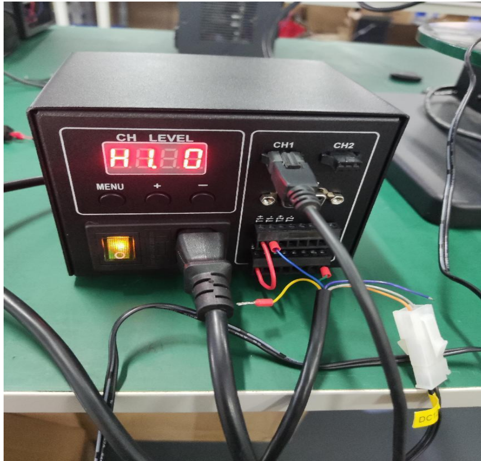
Figure 17: Set to External Trigger Mode
