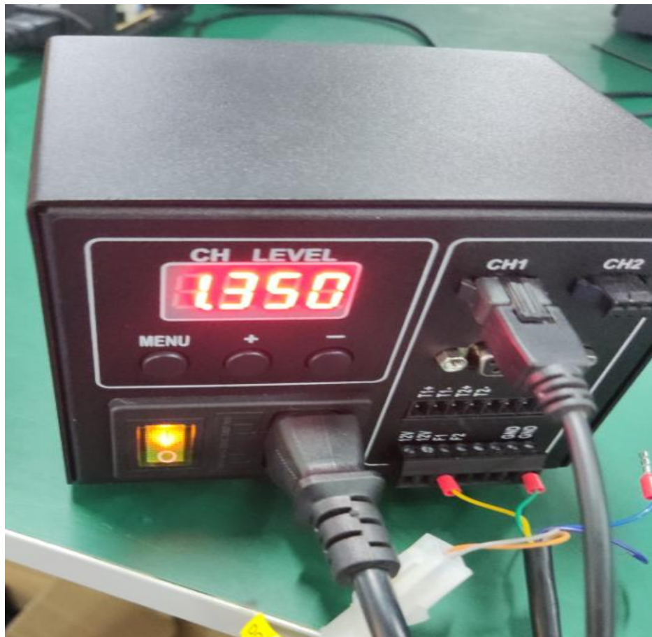
Figure 20: Strobe Time Setting and Wiring Method
