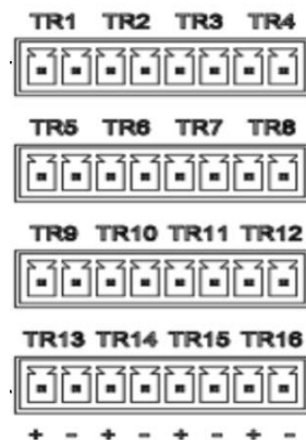
Figure 3 External Trigger Input Interface
